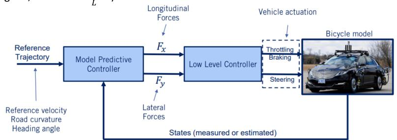
MPC for dynamic vehicle model (high-level controller) with forces (longitudinal and lateral) as control input.
