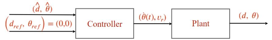
PID controller for kinematic bicycle model with heading angle rate  $(\dot{\theta})$  and velocity  $(v_r,$  constant here) as control input. ( $\dot{\theta}$  should be controlled indirectly by controlling steering angle  $\delta$ , with  $\dot{\theta} = \frac{v \tan \delta}{L}$ .)
