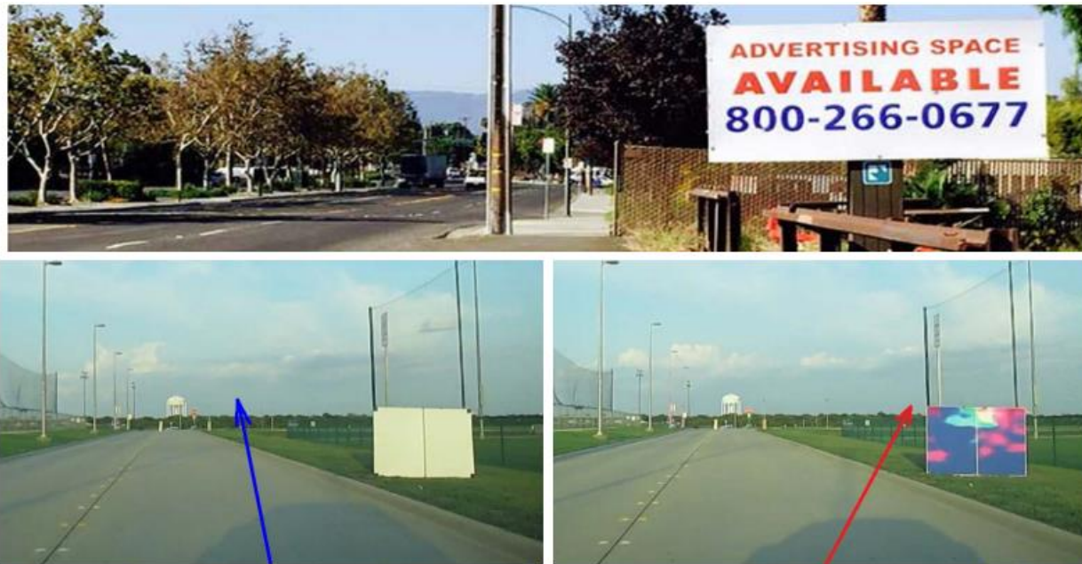
Figure 1: The top subfigure shows an example customizable roadside billboard. The bottom two subfigures show an adversarial billboard example, where the Dave [4] steering model diverges under our proposed approach.
