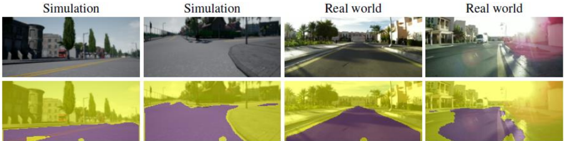
Figure 7: Sample outputs of the segmentation network trained on Cityscapes and tested in simulation and in the real world. The images are at the resolution used by the network – 200 \times 88 pixels. The network works well in typical scenes both in simulation and in the real world, but accuracy drops under complex lighting conditions and in unusual situations.
