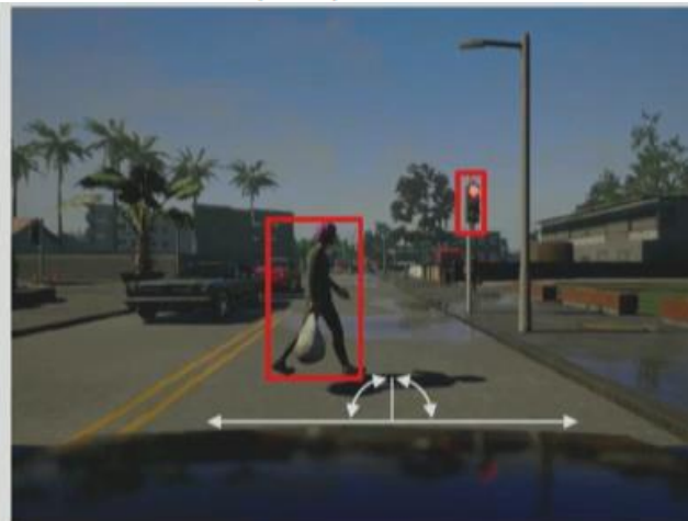
Figure 3: Affordances. Left: We categorize affordances according to their type (discrete/continuous) and whether they are conditional (dependent on directional input) or unconditional. Right: Illustration of the affordances (red) and observation areas used by our model.
